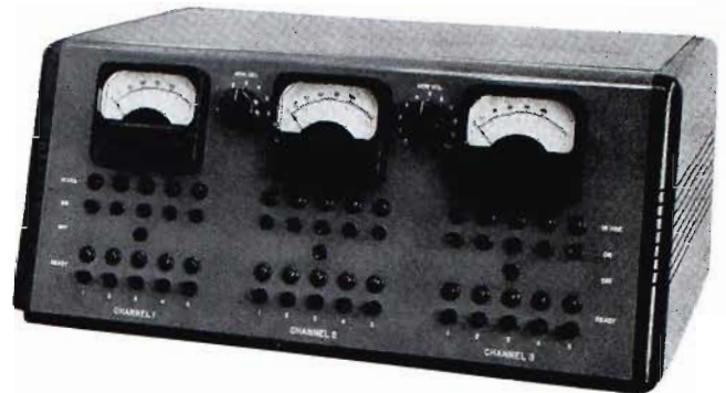
Master Switching Console
